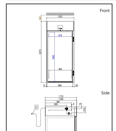
ΕI Electrical inlet (power) Refrigerant Inlet RO Refrigerant Outlet
